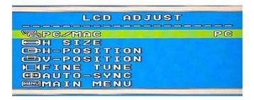
**PC/MAC** Switches between PC at 800X600 resolution and MAC at 832X624 resolution. Select PC/MAC, using [+] or [–] button. Then press [Menu] to initiate the switch between PC and MAC shown as above. Note: This function is to support MAC 832 x 624 resolution only.
